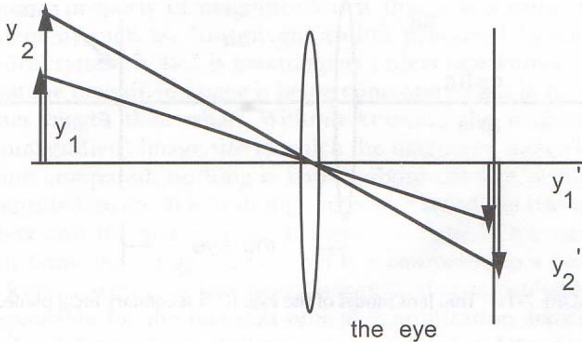
FIGURE 7-4. Relative size magnification. ( $y_1$  = original object size;  $y_2$  = new object size;  $y_1'$  = image size of object  $y_1$ ;  $y_2'$  = image size of object  $y_2$ .)
